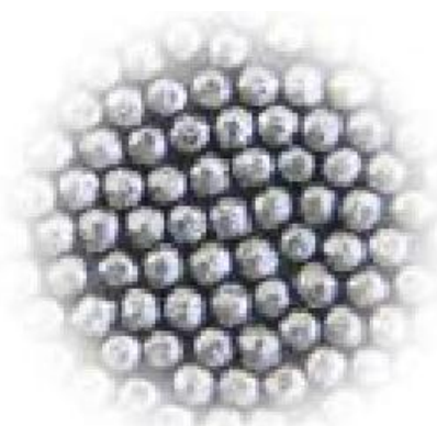
G3 (spherical grain)
