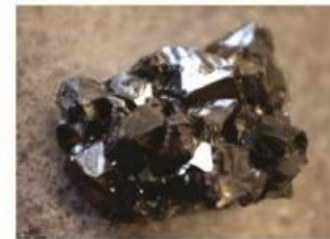
Fig. 6. Absorption of light of different wavelengths by sphalerite, which result in colours ranging from clear, honey yellow (cleiophane) to black (marmatite) as the concentration of iron in the sphalerite increases. (a) Band structure showing the iron bands within the bandgap. (b) Absorption spectrum of a sphalerite sample containing 7% iron (Wincott and Vaughan, 2006). (c) Samples of cleiophane (orange/red) and marmatite (black). (For interpretation of the references to color in this figure legend, the reader is referred to the web version of this article.)
