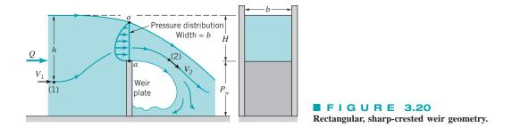
For now, we will take a very simple approach and assume that the weir flow is similar in many respects to an orifice-type flow with a free streamline. In this instance we would expect the average velocity across the top of the weir to be proportional to  $\sqrt{2gH}$  and the flow area for this rectangular weir to be proportional to *Hb*. Hence, it follows that
