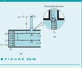
Since  $V_1 = V_2 = V_0$  and  $z_1 = z_2 = 0$ , it follows that  $p_1 = p_2 = p_0$ and the Bernoulli constant for this streamline,  $C_{12}$ , is given by
