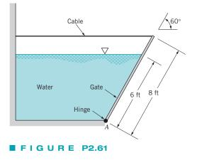
in Fig. P2.61. Water acts against the gate which is hinged at point *A*. Friction in the hinge is negligible. Determine the tension in the cable.
