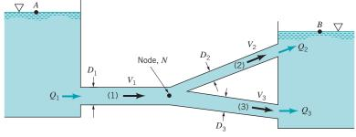
FIGURE 8.36 Multiple pipe loop system.
