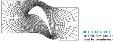
**FIGURE A.5** Finite difference grid for flow past a turbine blade. (From Ref. 9, used by permission.)
