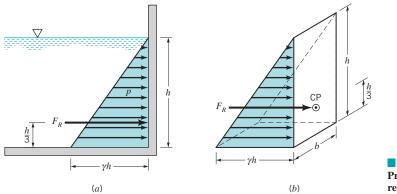
**FIGURE 2.19** Pressure prism for vertical rectangular area.
