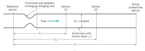
(b) **FIGURE 11.20** (a) Unchoked Fanno flow. (b) Choked Fanno flow.
