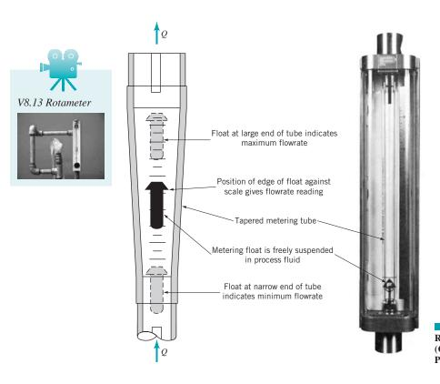
**FIGURE 8.46** Rotameter-type flow meter. (Courtesy of Fischer & Porter Co.)
