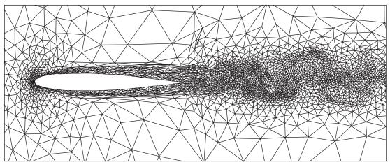
■ F I G U R E A.4 Anisotropic adaptive mesh for the calculation of viscous flow over a NACA 0012 airfoil at a Reynolds number of 10,000, Mach number of 0.755, and angle of attack of 1.5°. (From CFD Laboratory, Concordia University, Montreal, Canada. Used by permission.)
