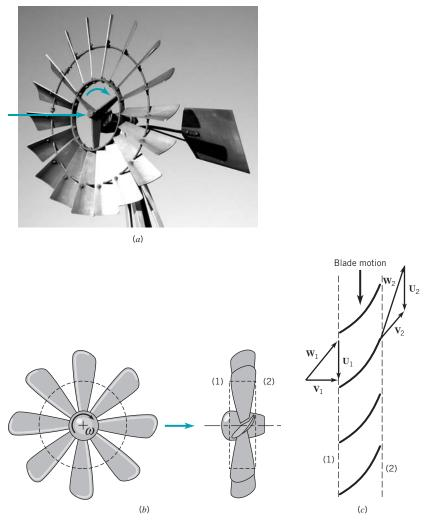
**FIGURE 12.4** Idealized flow through a windmill: (a) windmill; (b) windmill blade geometry; (c) absolute velocity, V; relative velocity, W; and blade velocity, U; at the inlet and exit of the windmill blade section.
