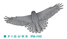
alter their body shape and increase their planform area, *A*, by spreading their wing and tail feathers, thereby reducing their flight speed. If during landing the planform area is increased by 50% and the lift coefficient increased by 30% while all other parameters are held constant, by what percent is the flight speed reduced?
