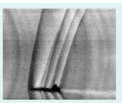
**FIGURE E11.4***b* NASA Schlieren photograph of shock waves from a T-38 aircraft at Mach 1.1, 13,000 feet.
