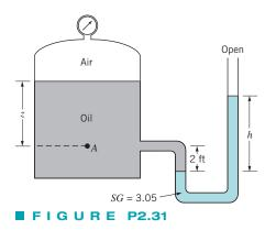
the tank is oil ( $\gamma = 54.0 \text{ lb/ft}^3$ ). The pressure at point *A* is 2.00 psi. Determine: (a) the depth of oil, *z*, and (b) the differential reading, *h*, on the manometer.
