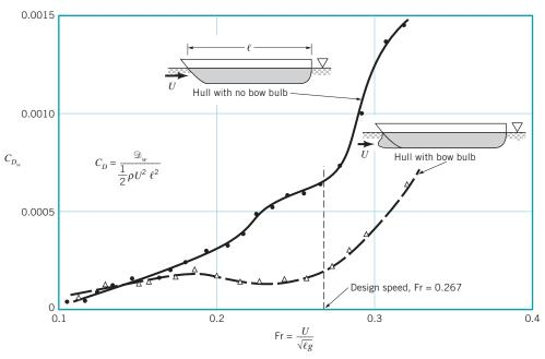
**FIGURE 9.26** Typical drag coefficient data as a function of Froude number and hull characteristics for that portion of the drag due to the generation of waves (adapted from Ref. 25).
