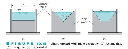
A sharp-crested weir can be used to determine the flowrate.
