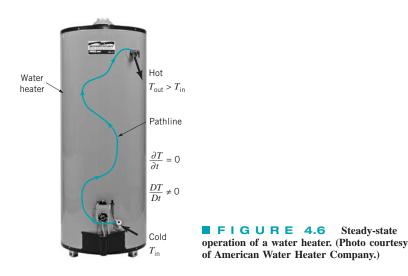
The convective derivative is a result of the spatial variation of the flow. It is due to the convection, or motion, of the particle through space in which there is a gradient  $[\nabla() = \partial()/\partial x \,\hat{\mathbf{i}} + \partial()/\partial y \,\hat{\mathbf{j}} + \partial()/\partial z \,\hat{\mathbf{k}}]$  in the parameter value. That portion of the acceleration given by the term  $(\mathbf{V} \cdot \nabla)\mathbf{V}$  is termed the *convective acceleration*.
