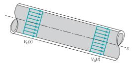
**FIGURE 4.5** Uniform, unsteady flow in a constant diameter pipe.
