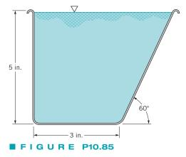
during a heavy rain storm. The cross section of the gutter is shown in Fig. P10.85. Determine the vertical distance that this gutter must be pitched (i.e., the difference in elevation between the two ends of the gutter) so that the water does not overflow the gutter. Assume uniform depth channel flow.
