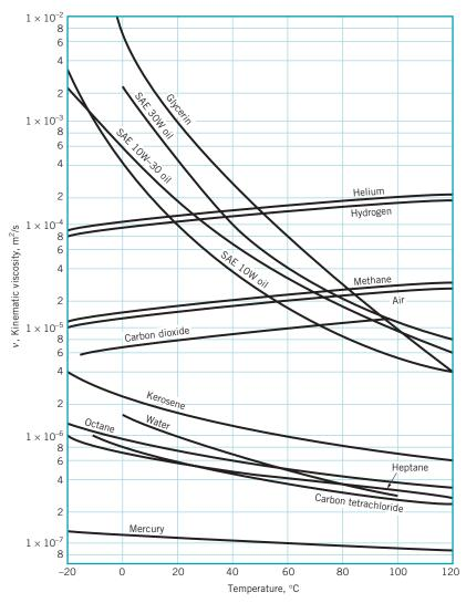
**FIGURE B.2** Kinematic viscosity of common fluids (at atmospheric pressure) as a function of temperature. To convert to BG units of ft<sup>2</sup>/s multiply m<sup>2</sup>/s by 10.76. (Curves from R. W. Fox and A. T. McDonald, *Introduction to Fluid Mechanics*, 3rd Ed., Wiley, New York, 1985. Used by permission.)
