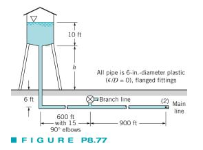
and the branch line is shut off. Determine the minimum height, h, of the water tank under the assumption that (a) minor losses are negligible, (b) minor losses are not negligible.
