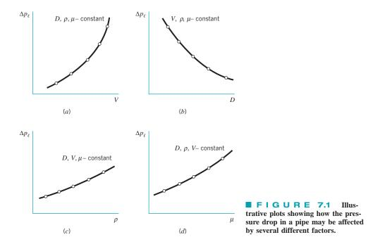
Dimensionless products are important and useful in the planning, execution, and interpretation of experiments. original list of variables, as described in Eq. 7.1, we can collect these into two nondimensional combinations of variables (called *dimensionless products* or *dimensionless groups*) so that
