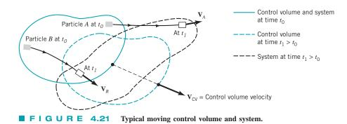
The absolute and relative velocities differ by an amount equal to the control volume velocity.
