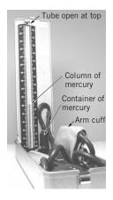
The simplest type of manometer consists of a vertical tube, open at the top, and attached to the container in which the pressure is desired, as illustrated in Fig. 2.9. The figure in the margin shows an important device whose operation is based upon this principle. It is a sphygmomanometer, the traditional instrument used to measure blood pressure.
