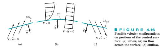
The flowrate of a parameter across the control surface is written in terms of a surface integral.
