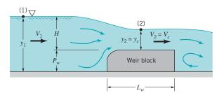
**FIGURE 10.23** Broad-crested weir geometry.
