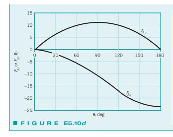
to the left ( $F_{Ax}$  is negative) and up in order to change the direction of flow of the water from horizontal to vertical. This momentum change requires a force. If  $\theta = 180^\circ$ , the water jet is turned back on itself. This requires no vertical force ( $F_{Az} = 0$ ), but the horizontal force ( $F_{Ax} = -23.3$  lb) is two times that required if  $\theta = 90^\circ$ . This horizontal fluid momentum change requires a horizontal force only.
