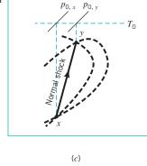
**FIGURE 11.26** (*a*) The normal shock in a Fanno flow. (*b*) The normal shock in a Rayleigh flow. (*c*) The normal shock in a frictionless and adiabatic flow.
