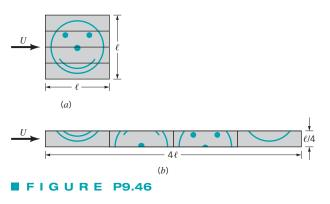
**9.47** If the drag on one side of a flat plate parallel to the upstream flow is  $\mathfrak{D}$  when the upstream velocity is *U*, what will the drag be when the upstream velocity is 2*U*; or *U*/2? Assume laminar flow.
