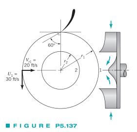
flow leaving the rotor at section (2) is without angular momentum. If the flowing fluid is air and the static pressure drop across the rotor is 0.01 psi, determine the loss of available energy across the rotor and the rotor aerodynamic efficiency.
