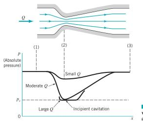
**FIGURE 3.16** Pressure variation and cavitation in a variable area pipe.
