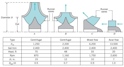
**FIGURE 12.21** Comparison of different types of impellers. Specific speed for centrifugal pumps based on single suction and identical flowrate. (Adapted from Ref. 12, used with permission.)
