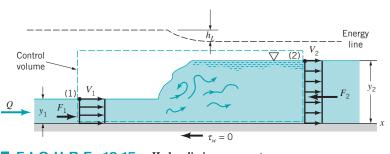
**FIGURE 10.15** Hydraulic jump geometry.
