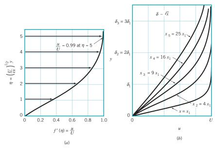
**FIGURE 9.10** Blasius boundary layer profile: (a) boundary layer profile in dimensionless form using the similarity variable  $\eta$ , (b) similar boundary layer profiles at different locations along the flat plate.
