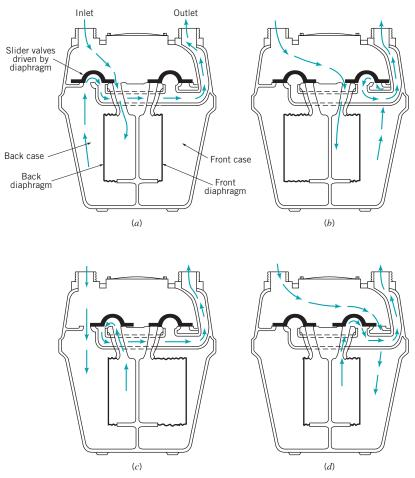
**FIGURE 8.49** Bellows-type flow meter. (Courtesy of BTR—Rockwell Gas Products). (a) Back case emptying, back diaphragm filling. (b) Front diaphragm filling, front case emptying. (c) Back case filling, back diaphragm emptying. (d) Front diaphragm emptying, front case filling.
