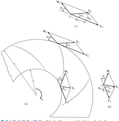
**FIGURE 12.8** Vel centrifugal pump impeller.
