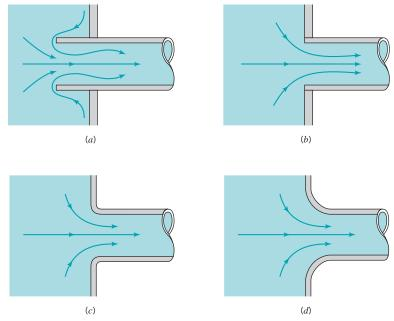
**FIGURE 8.22** Entrance flow conditions and loss coefficient (Refs. 28, 29). (a) Reentrant,  $K_L = 0.8$ , (b) sharp-edged,  $K_L = 0.5$ , (c) slightly rounded,  $K_L = 0.2$  (see Fig. 8.24), (d) well-rounded,  $K_L = 0.04$  (see Fig. 8.24).
