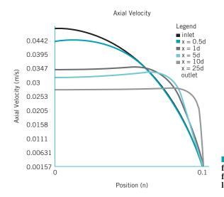
**FIGURE A.2** Entrance flow in a pipe. Velocity profiles as a function of radial position for various locations along the pipe length.
