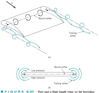
■ **F I G U R E 9.37** Flow past a finite length wing: (*a*) the horseshoe vortex system produced by the bound vortex and the trailing vortices; (*b*) the leakage of air around the wing tips produces the trailing vortices.
