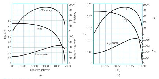
**FIGURE 12.17** Typical performance data for a centrifugal pump: (*a*) characteristic curves for a 12-in. centrifugal pump operating at 1000 rpm, (*b*) dimensionless characteristic curves. (Data from Ref. 8, used by permission.)
