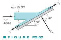
is 30 mm. If the air velocity magnitude remains constant as the air flows over the plate surface in the directions shown, determine: (a) the magnitude of  $F_{A_1}$  the anchoring force required to hold the plate stationary; (b) the fraction of mass flow along the plate surface in each of the two directions shown; (c) the magnitude of  $F_{A_1}$  the anchoring force required to allow the plate to move to the right at a constant speed of 10 m/s.
