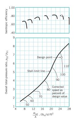
**FIGURE 12.37** Performance characteristics of an axial-flow compressor (Ref. 19).
