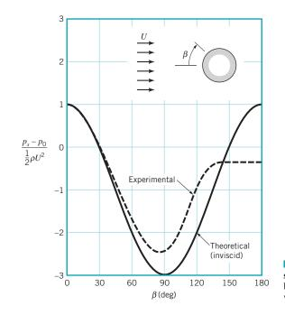
■ **FIGURE 6.27** A comparison of theoretical (inviscid) pressure distribution on the surface of a circular cylinder with typical experimental distribution.
