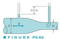
**3.54** A 0.15-m-diameter pipe discharges into a 0.10-m-diameter pipe. Determine the velocity head in each pipe if they are carrying  $0.12 \text{ m}^3$ /s of kerosene.
