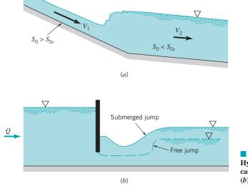
**FIGURE 10.17** Hydraulic jump variations: (*a*) jump caused by a change in channel slope, (*b*) submerged jump.
