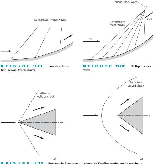
**FIGURE 11.33** Supersonic flow over a wedge: (*a*) Smaller wedge angle results in attached oblique shock. (*b*) Large wedge angle results in detached curved shock.
