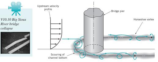
**FIGURE** 10.14 The complex three-dimensional flow structure around a bridge pier.
