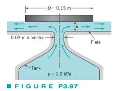
effects and elevation changes are assumed negligible and the flow exits radially from the circumference of the circular disk with uniform velocity.
