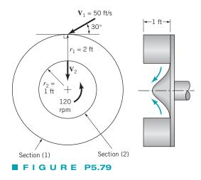
**5.79** A water turbine with radial flow has the dimensions shown in Fig.P5.79.The absolute entering velocity is 50 ft/s, and it makes an
