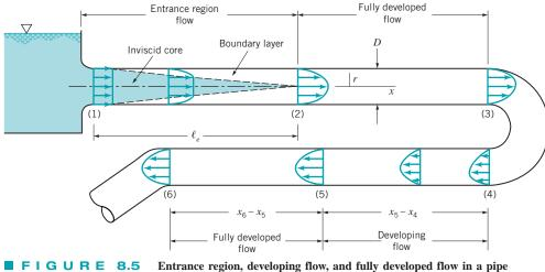
**FIGURE 8.5** Entrance region, developing flow, and fully developed flow in a pip system.
