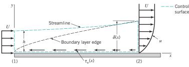
**FIGURE 9.11** Control volume used in the derivation of the momentum integral equation for boundary layer flow.
