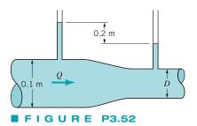
**3.53** Water flows through the pipe contraction shown in Fig. P3.53. For the given 0.2-m difference in the manometer level, determine the flowrate as a function of the diameter of the small pipe, D.
