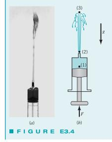
plunger will produce a pressure greater than atmospheric at point (1) within the syringe. The water flows from the needle, point (2), with relatively high velocity and coasts up to point (3) at the top of its trajectory.
