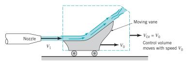
**FIGURE 4.20** Example of a moving control volume.
