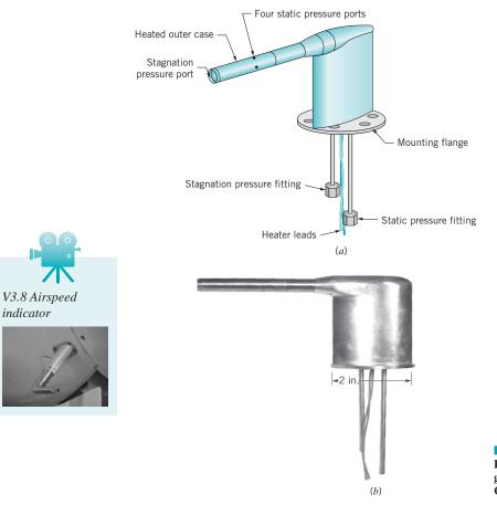
**FIGURE 3.7** Airplane Pitot-static probe. (a) Schematic, (b) Photograph, (Photograph courtesy of SpaceAge Control, Inc.)
