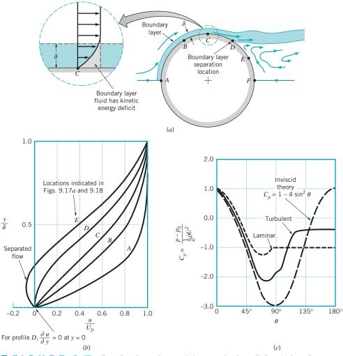
**FIGURE 9.17** Boundary layer characteristics on a circular cylinder: (*a*) boundary layer separation location, (*b*) typical boundary layer velocity profiles at various locations on the cylinder, (*c*) surface pressure distributions for inviscid flow and boundary layer flow.
