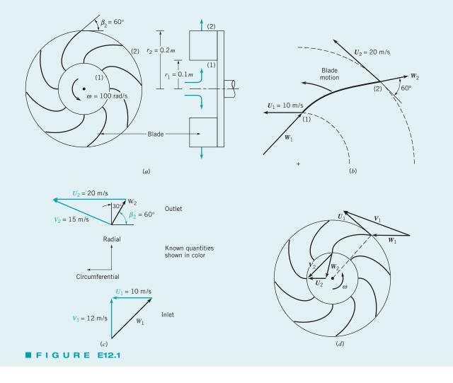
**COMMENT** On the other hand, by reversing the direction of flow from larger to smaller radii, this device can become a radial-flow turbine. In this case (Fig. E12.1*d*) the flow direction is reversed (compared to that in Figs. E12.1*a*, *b*, and *c*) and the velocity triangles are as indicated. Stationary vanes around the perimeter of the rotor would be needed to achieve  $V_1$  as shown. Note that the component of the absolute velocity, V, in the di-
