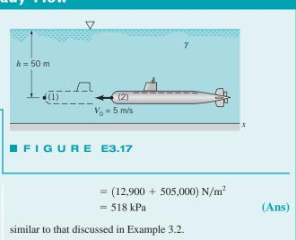
**COMMENT** If the submarine were accelerating,  $\partial V_0 / \partial t \neq 0$ , the flow would be unsteady in either of the above coordinate systems and we would be forced to use an unsteady form of the Bernoulli equation.
