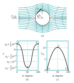
**FIGURE 9.16** Inviscid flow past a circular cylinder: (*a*) streamlines for the flow if there were no viscous effects, (*b*) pressure distribution on the cylinder's surface, (*c*) free-stream velocity on the cylinder's surface.
