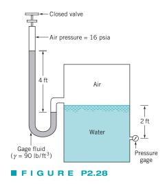
manometer the air pressure is 16 psia. Determine the reading on the pressure gage for a differential reading of 4 ft on the manometer. Express your answer in psi (gage). Assume standard atmospheric pressure and neglect the weight of the air columns in the manometer.
