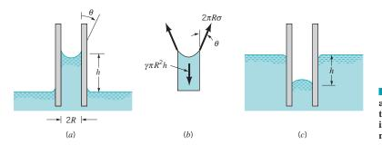
**FIGURE 1.10** Effect of capillary action in small tubes. (*a*) Rise of column for a liquid that wets the tube. (*b*) Free-body diagram for calculating column height. (*c*) Depression of column for a nonwetting liquid.
