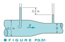
**3.52** Water flows through the pipe contraction shown in Fig. P3.52. For the given 0.2-m difference in the manometer level, determine the flowrate as a function of the diameter of the small pipe, *D*.
