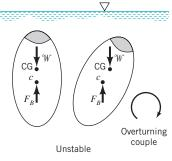
**FIGURE 2.26** Stability of a completely immersed body—center of gravity above centroid.
