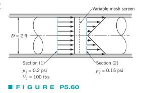
2-ft-diameter circular cross section duct. The static pressures upstream and downstream of the screen are 0.2 and 0.15 psi and are uniformly distributed over the flow cross section area. Neglecting the force exerted by the duct wall on the flowing air, calculate the screen drag force.
