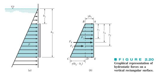
This same graphical approach can be used for plane rectangular surfaces that do not extend up to the fluid surface, as illustrated in Fig. 2.20*a*. In this instance, the cross section of the pressure prism is trapezoidal. However, the resultant force is still equal in magnitude to the volume of the pressure prism, and it passes through the centroid of the volume. Specific values can be obtained by decomposing the pressure prism into two parts, *ABDE* and *BCD*, as shown in Fig. 2.20*b*. Thus,
