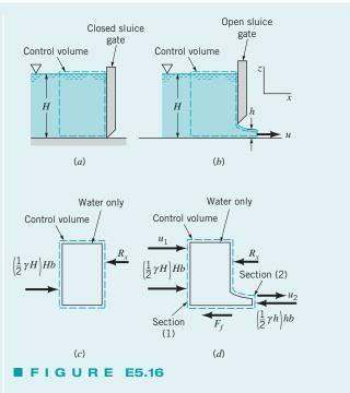
If  $H \ge h$ , the upstream velocity,  $u_1$ , is much less than  $u_2$  so that the contribution of the incoming momentum flow to the control surface integral can be neglected and from Eq. 5 we obtain
