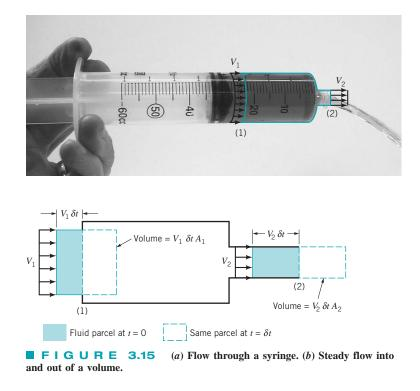
$V_2 = A_1V_1/A_2 = 2V_1$ . The use of the Bernoulli equation and the flowrate equation (continuity equation) is demonstrated by Example 3.7.
