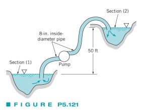
energy associated with 2.5 ft<sup>3</sup>/s being pumped from sections (1) to (2) is  $loss = 61\overline{V}^{2}/2$  ft<sup>2</sup>/s<sup>2</sup>, where  $\overline{V}$  is the average velocity of water in the 8-in. inside diameter piping involved. Determine the amount of shaft power required.
