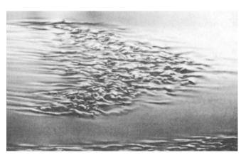
■ FIGURE 9.13 Turbulent spots and the transition from laminar to turbulent boundary layer flow on a flat plate. Flow from left to right. (Photograph courtesy of B. Cantwell, Stanford University.)
