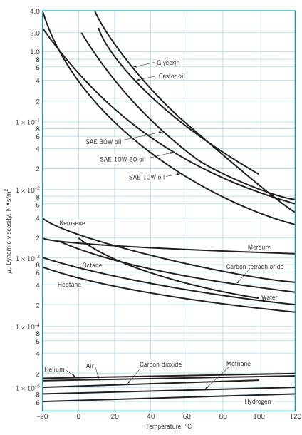
**FIGURE B.1** Dynamic (absolute) viscosity of common fluids as a function of temperature. To convert to BG units of  $lb \cdot s/ft^2$  multiply N  $\cdot s/m^2$  by 2.089  $\times 10^{-2}$ . (Curves from R. W. Fox and A. T. McDonald, *Introduction to Fluid Mechanics*, 3rd Ed., Wiley, New York, 1985. Used by permission.)
