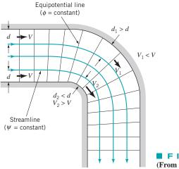
**FIGURE 6.15** Flow net for a 90° bend. (From Ref. 3, used by permission.)
