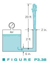
**3.39** An inviscid, incompressible liquid flows steadily from the large pressurized tank shown in Fig. P.3.39. The velocity at the exit is 40 ft/s. Determine the specific gravity of the liquid in the tank.
