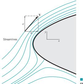
**FIGURE 6.7** Velocity and velocity components along a streamline.
