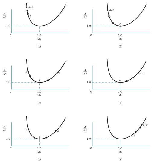
**FIGURE 11.11** (*a*) Subsonic to subsonic isentropic flow (not choked). (*b*) Subsonic to subsonic isentropic flow (choked). (*c*) Subsonic to supersonic isentropic flow (choked). (*d*) Supersonic to supersonic isentropic flow (choked). (*e*) Supersonic to subsonic isentropic flow (choked). (*f*) Supersonic to supersonic isentropic flow (not choked).
