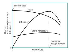
**FIGURE 12.11** Typical performance characteristics for a centrifugal pump of a given size operating at a constant impeller speed.
