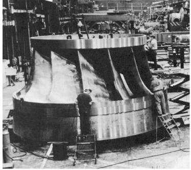
(b) **FIGURE 12.23** (a) Schematic diagram of a reaction turbine, (b) photograph of a reaction turbine. (Courtesy of Voith Hydro, York, PA.)
