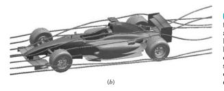
**FIGURE 9.1** (*a*) Flow past a full-sized streamlined vehicle in the GM aerodynamics laboratory wind tunnel, an 18-ft by 34-ft test section facility driven by a 4000-hp, 43-ft-diameter fan. (Photograph courtesy of General Motors Corporation.) (*b*) Predicted streamlines for flow past a Formula 1 race car as obtained by using computational fluid dynamics techniques. (Courtesy of Ansys, Inc.)
