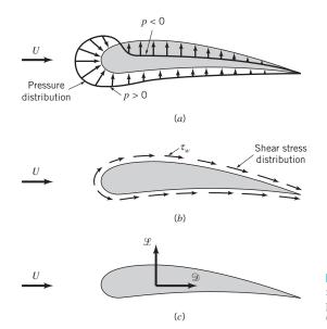
■ **FIGURE 9.3** Forces from the surrounding fluid on a two-dimensional object: (*a*) pressure force, (*b*) viscous force, (*c*) resultant force (lift and drag).
