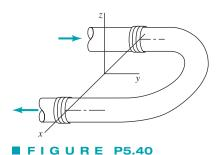
The pressures at the entrance and exit of the bend are 210 and 165 kPa, respectively. Calculate the horizontal (x and y) components of the anchoring force needed to hold the bend in place.
