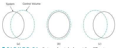
**FIGURE 5.1** System and control volume at three different instances of time. (a) System and control volume at time  $t - \delta t$ . (b) System and control volume at time t, coincident condition. (c) System and control volume at time  $t + \delta t$ .
