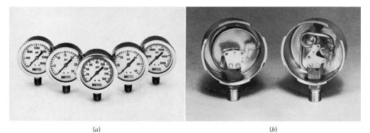
**FIGURE 2.13** (a) Liquid-filled Bourdon pressure gages for various pressure ranges. (b) Internal elements of Bourdon gages. The "C-shaped" Bourdon tube is shown on the left, and the "coiled spring" Bourdon tube for high pressures of 1000 psi and above is shown on the right. (Photographs courtesy of Weiss Instruments, Inc.)
