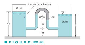
reservoir on the left, which contains carbon tetrachloride, is closed and pressurized to 8 psi. The reservoir on the right contains water and is open to the atmosphere. With the given data, determine the depth of water, h, in the right reservoir.
