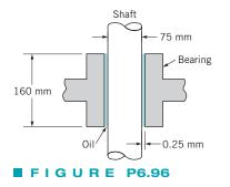
**6.97** A viscous fluid is contained between two long concentric cylinders. The geometry of the system is such that the flow between the cylinders is approximately the same as the laminar flow between two infinite parallel plates. (a) Determine an expression for the torque required to rotate the outer cylinder with an angular velocity  $\omega$ .
