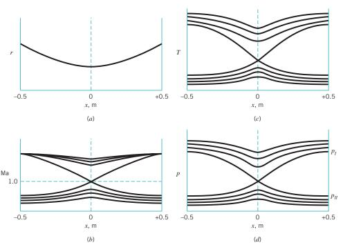
**FIGURE 11.12** (a) The variation of duct radius with axial distance. (b) The variation of Mach number with axial distance. (c) The variation of temperature with axial distance. (d) The variation of pressure with axial distance.
