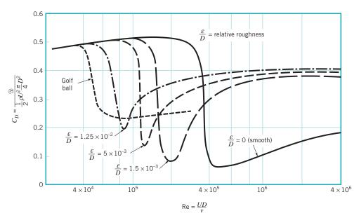
**FIGURE 9.25** The effect of surface roughness on the drag coefficient of a sphere in the Reynolds number range for which the laminar boundary layer becomes turbulent (Ref. 5).
