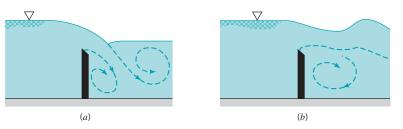
**FIGURE 10.22** Flow conditions over a weir without a free nappe: (*a*) plunging nappe, (*b*) submerged nappe.
