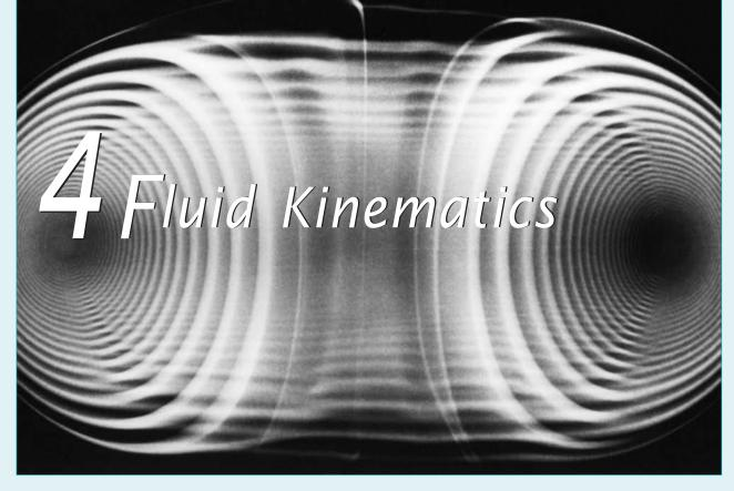
CHAPTER OPENING PHOTO: A vortex ring: The complex, three-dimensional structure of a smoke ring is indicated in this cross-sectional view. (Smoke in air.) [Photograph courtesy of R. H. Magarvey and C. S. MacLatchy (Ref. 4).]
