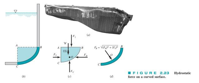
The resultant  $F_R$  passes through the point O, which can be located by summing moments about an appropriate axis. The resultant force of the fluid acting *on the curved surface BC* is equal and opposite in direction to that obtained from the free-body diagram of Fig. 2.23*c*. The desired fluid force is shown in Fig. 2.23*d*.
