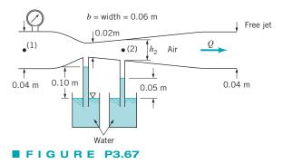
**3.68** Water flows steadily from the large open tank shown in Fig. P3.68. If viscous effects are negligible, determine (a) the flowrate, Q, and (b) the manometer reading, h.
