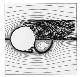
**FIGURE A.8** Streamlines for flow past a circular cylinder at a short time after the flow was impulsively started. The upper half is a photograph from a flow visualization experiment. The lower half is from a finite difference calculation. (See the photograph at the beginning of Chapter 9.) (From Ref. 9, used by permission.)
