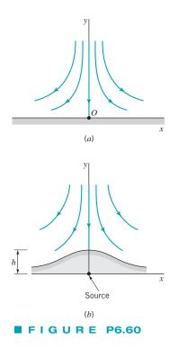
**6.61** The combination of a uniform flow and a source can be used to describe flow around a streamlined body called a half-body. (See **Video V6.5.**) Assume that a certain body has the shape of a half-body with a thickness of 0.5 m. If this body is placed in an airstream moving at 15 m/s, what source strength is required to simulate flow around the body?
