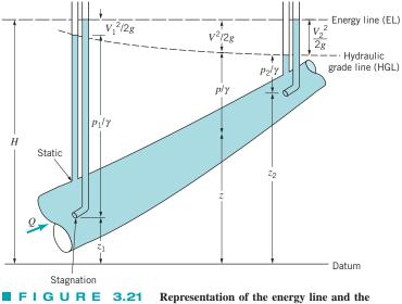
**FIGURE 3.21** Representation of the energy line and th hydraulic grade line.
