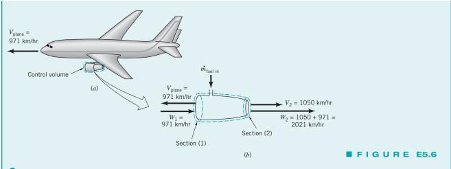
The control volume, which moves with the airplane (see Fig. E5.6b), surrounds the engine and its contents and includes all fluids involved at an instant. The application of Eq. 5.16 to these contents of the control volume yields
