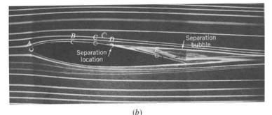
**FIGURE 9.18** Flow visualization photographs of flow past an airfoil (the boundary layer velocity profiles for the points indicated are similar to those indicated in Fig. 9.17*b*): (*a*) zero angle of attack, no separation, (*b*) 5° angle of attack, flow separation. Dye in water. (Photograph courtesy of ONERA, France.)
