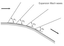
**FIGURE 11.27** Flow acceleration across a Mach wave.
