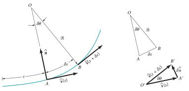
**FIGURE 4.9** Relationship between the unit vector along the streamline,  $\hat{s}$ , and the radius of curvature of the streamline,  $\Re$ .
