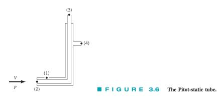
where p and V are the pressure and velocity of the fluid upstream of point (2). The outer tube is made with several small holes at an appropriate distance from the tip so that they measure the static pressure. If the effect of the elevation difference between (1) and (4) is negligible, then
