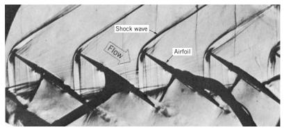
**FIGURE 11.4** The Schlieren visualization of flow (supersonic to subsonic) through a row of compressor airfoils. (Photograph provided by Dr. Hans Starken, Germany.)
