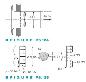
pipe exit the velocity is nonuniform as indicated. The shear stress along the pipe wall is negligible. (a) Determine the head loss associated with a particle as it flows from the uniform velocity upstream of the object to a location in the wake at the exit plane of the pipe. (b) Determine the force that the air puts on the object.
