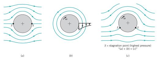
**FIGURE 9.38** Inviscid flow past a circular cylinder: (*a*) uniform upstream flow without circulation, (*b*) free vortex at the center of the cylinder, (*c*) combination of free vortex and uniform flow past a circular cylinder giving nonsymmetric flow and a lift.
