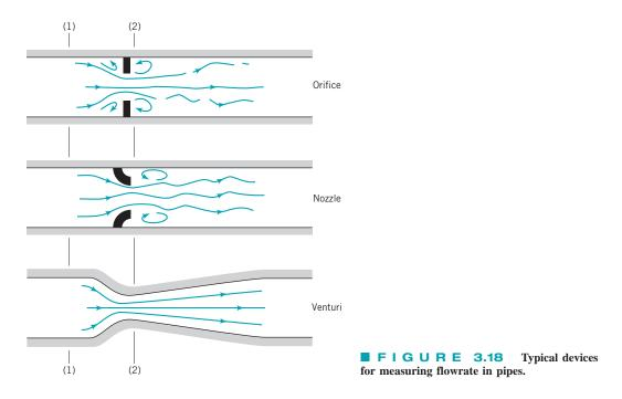
conduits and devices to measure flowrates in open channels. In this chapter we will consider "ideal" *flow meters*—those devoid of viscous, compressibility, and other "real-world" effects. Corrections for these effects are discussed in Chapters 8 and 10. Our goal here is to understand the basic operating principles of these simple flow meters.
