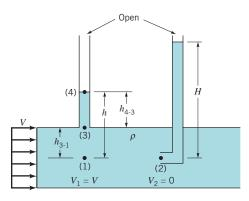
**FIGURE 3.4** Measurement of static and stagnation pressures.
