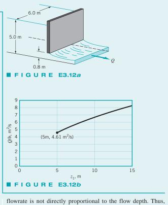
for example, if during flood conditions the upstream depth doubled from  $z_1 = 5$  m to  $z_1 = 10$  m, the flowrate per unit width of the channel would not double, but would increase only from 4.61 m<sup>2</sup>/s to 6.67 m<sup>2</sup>/s.
