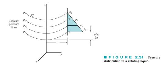
The free surface in a rotating liquid is curved rather than flat.
