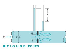
**<sup>8.124</sup>** Water flows through the orifice meter shown in Fig. P8.123 such that h = 1.6 ft with d = 1.5 in. Determine the flowrate.
