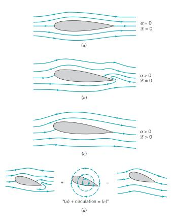
■ **FIGURE 9.36** Inviscid flow past an airfoil: (*a*) symmetrical flow past the symmetrical airfoil at a zero angle of attack; (*b*) same airfoil at a nonzero angle of attack—no lift, flow near trailing edge not realistic; (*c*) same conditions as for (*b*) except circulation has been added to the flow—nonzero lift, realistic flow; (*d*) superposition of flows to produce the final flow past the airfoil.
