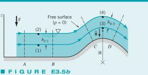
the inviscid, incompressible, steady flow shown in Fig. E3.5*b*. From section *A* to *B* the streamlines are straight, while from *C* to *D* they follow circular paths.
