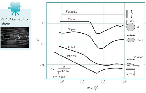
**FIGURE 9.22** Character of the drag coefficient as a function of Reynolds number for objects with various degrees of streamlining, from a flat plate normal to the upstream flow to a flat plate parallel to the flow (two-dimensional flow) (Ref. 5).
