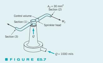
(a) We specify a control volume that contains the water in the rotary sprinkler head at any instant. This control volume is non-deforming, but it moves (rotates) with the sprinkler head.
