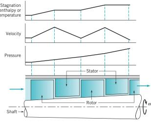
**FIGURE 12.35** Enthalpy, velocity, and pressure distribution in an axial-flow compressor.
