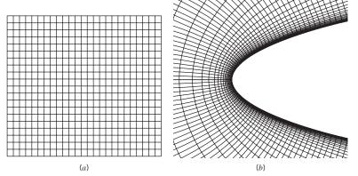
**FIGURE A.3** Structured grids. (*a*) Rectangular grid. (*b*) Grid around a parabolic surface.
