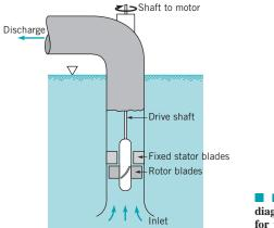
**FIGURE 12.19** Schematic diagram of an axial-flow pump arranged for vertical operation.
