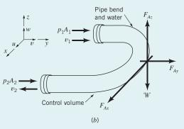
Note that the y component of velocity is positive at section (1) but is negative at section (2). Also, the mass flowrate term is negative at section (1) (flow in) and is positive at section (2) (flow out). From the continuity equation (Eq. 5.12), we get
