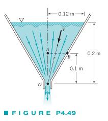
**4.50** Water flows though the slit at the bottom of a twodimensional water trough as shown in Fig. P4.50. Throughout most of the trough the flow is approximately radial (along rays from *O*) with a velocity of V = c/r, where *r* is the radial coordinate and *c* is a constant. If the velocity is 0.04 m/s when r = 0.1 m, determine the acceleration at points *A* and *B*.
