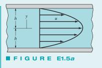
**COMMENT** From Eq. 2 we see that the velocity gradient (and therefore the shearing stress) varies linearly with y and in this particular example varies from 0 at the center of the channel to  $14.4 \text{ lb/ft}^2$  at the walls. This is shown in Fig. E1.5b. For the more general case the actual variation will, of course, depend on the nature of the velocity distribution.
