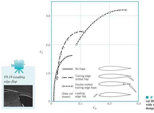
■ **FIGURE 9.35** Typical lift and drag alterations possible with the use of various types of flap designs (Ref. 21).
