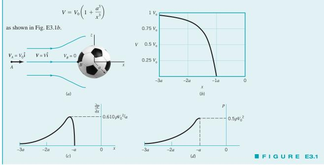
The net pressure force on a particle is determined by the pressure gradient.
