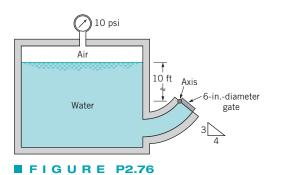
contains a spout that is closed by a 6-in.-diameter circular gate that is hinged along one side as illustrated. The horizontal axis of the hinge is located 10 ft below the water surface. Determine the minimum torque that must be applied at the hinge to hold the gate shut. Neglect the weight of the gate and friction at the hinge.
