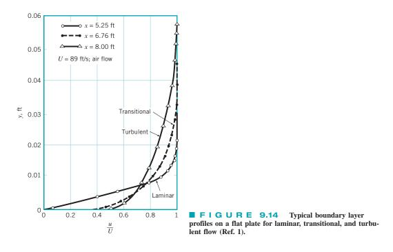
Transition from laminar to turbulent flow also involves a noticeable change in the shape of the boundary layer velocity profile. Typical profiles obtained in the neighborhood of the transition location are indicated in Fig. 9.14. The turbulent profiles are flatter, have a larger velocity gradient at the wall, and produce a larger boundary layer thickness than do the laminar profiles.
