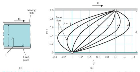
The viscous flow between parallel plates with bottom plate fixed and **FIGURE 6.32** upper plate moving (Couette flow): (a) coordinate system and notation used in analysis; (b) velocity distribution as a function of parameter, P, where  $P = -(b^2/2\mu U) \frac{\partial p}{\partial x}$ . (From Ref. 8, used by permission.)
