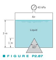
the tank has a specific weight of  $27 \text{ kN/m}^3$ . Determine the magnitude, direction, and line of action of the force exerted on the curved surface of the cone within the tank due to the 40-kPa pressure and the liquid.
