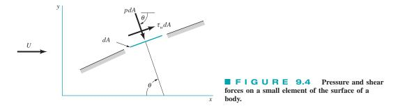
integrated or resultant effects of these distributions are needed. The resultant force in the direction of the upstream velocity is termed the *drag*,  $\mathfrak{D}$ , and the resultant force normal to the upstream velocity is termed the *lift*,  $\mathcal{L}$ , as is indicated in Fig. 9.3c. For some three-dimensional bodies there may also be a side force that is perpendicular to the plane containing  $\mathfrak{D}$  and  $\mathcal{L}$ .
