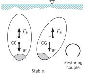
**FIGURE 2.25** Stability of a completely immersed body—center of gravity below centroid.
