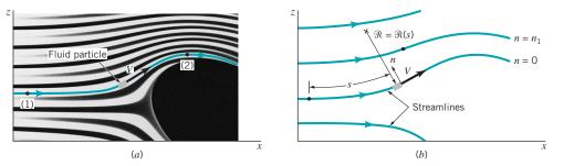
**FIGURE 3.1** (a) Flow in the x-z plane. (b) Flow in terms of streamline and normal coordinates.
