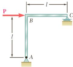
For the uniform rod and loading shown and using Castigliano's theorem, determine the deflection of 11 point B.
