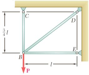
Knowing that the eight members of the indeterminate truss shown have the same uniform cross-14 sectional area, determine the force in member AB.
