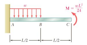
For the uniform beam shown, determine (a) the reaction at A, (b) the reaction at B. (use superposition method) 2
