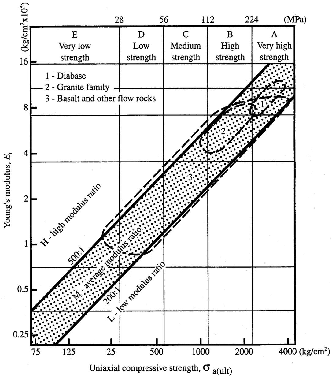
Figure 10-9a. Elastic Modulus-Compressive Strength Groupings for Intact Igneous Rock Materials (Deere & Miller, 1966).
