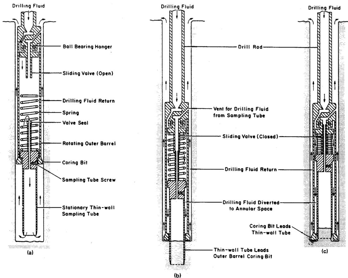
Figure 3-15: Pitcher Sampler. (a) Sampler Being Lowered into Drill Hole; (b) Sampler During Sampling of Soft Soils, (c) Sampler During Sampling of Stiff or Dense Soils. (Courtesy of Mobile Drilling, Inc.)
