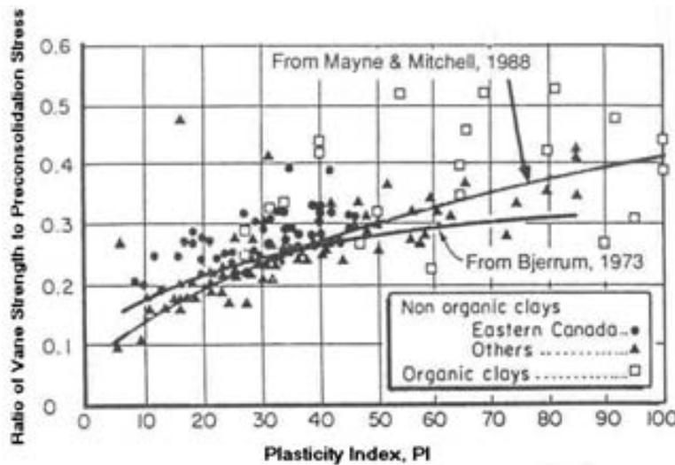
**Figure 9-19. Ratio of Measured Vane Strength to Preconsolidation Stress ( $s_{uv}/\sigma_p'$ ) vs. Plasticity Index ( $I_p$ ) (after Leroueil and Jamiolkowski, 1991)**
