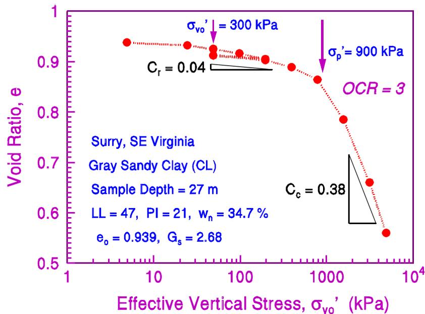
Figure 9-17. Representative Consolidation Test Results in Overconsolidated Clay
