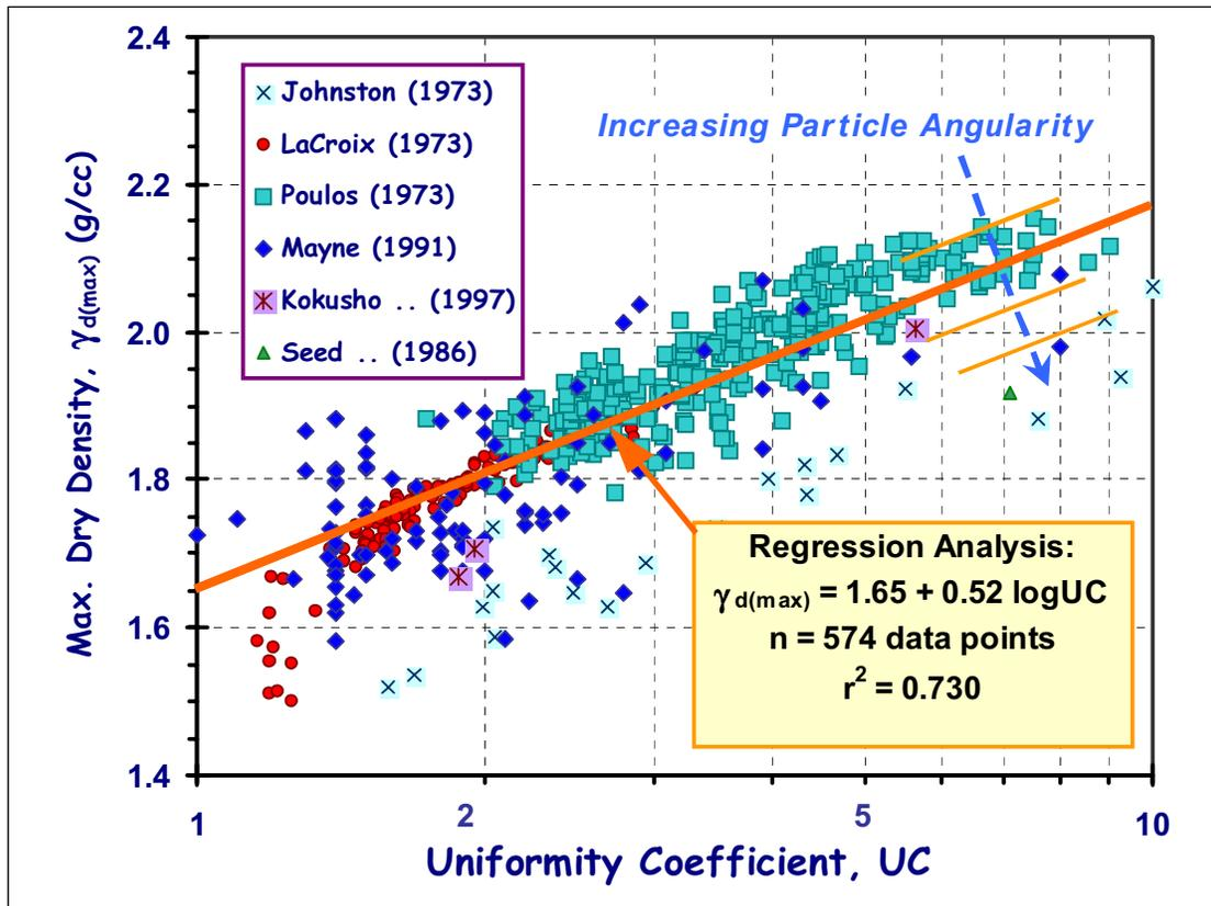
Figure 9-7. Maximum Dry Density Relationship with Sand Uniformity Coefficient ( $UC = D_{60}/D_{10}$ ).
