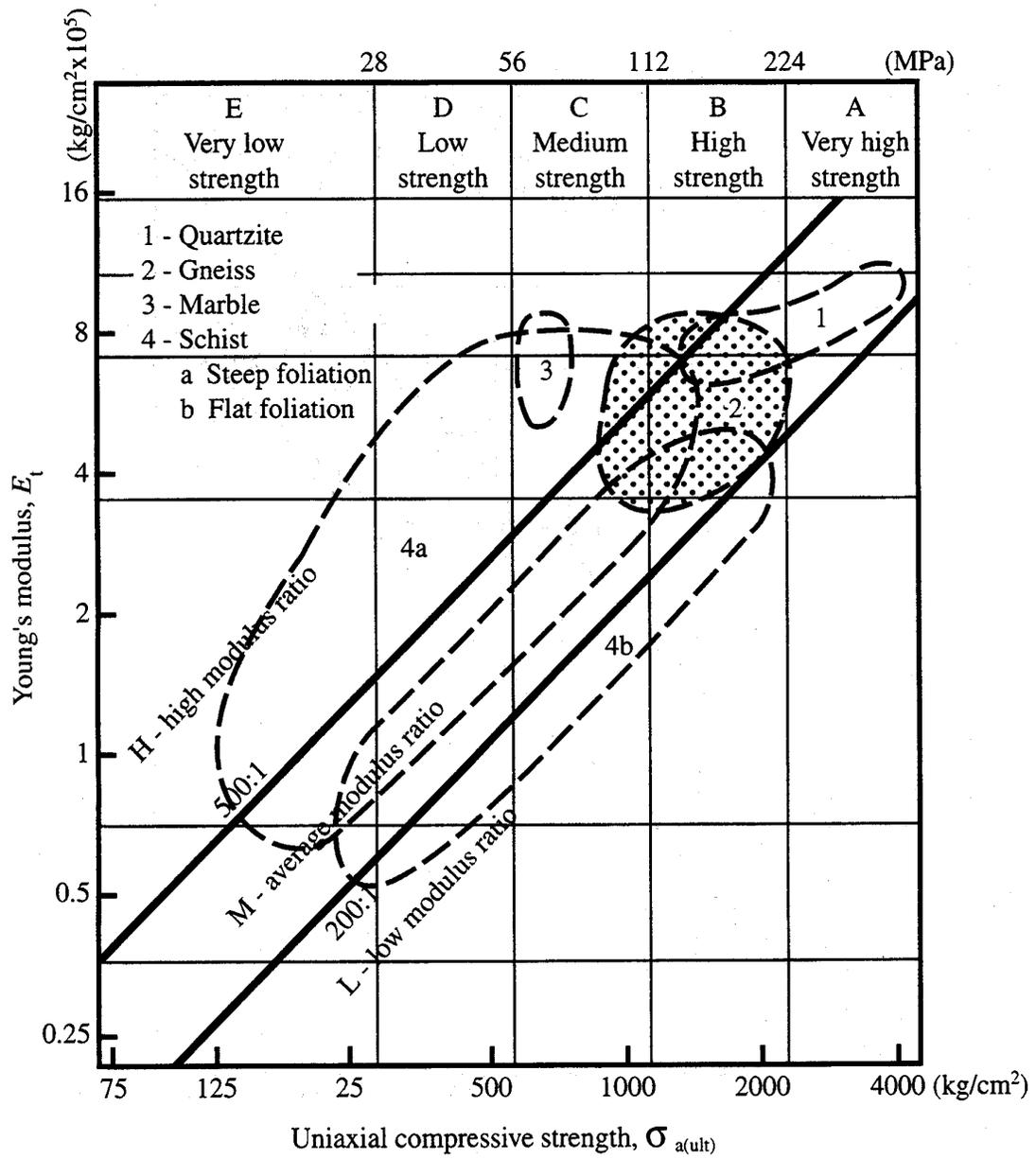
Figure 10-9c. Elastic Modulus-Compressive Strength Groupings for Intact Metamorphic Rock Materials (Deere & Miller, 1966).
