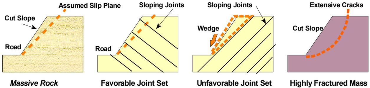
**Figure 10-11. Illustrative Cases for Defining Rock Shear Strength for Cut, including: (a) intact rock strength, (b) intact strength across joints, (c) shear strength along joint planes, and (d) jointed rock mass.**
