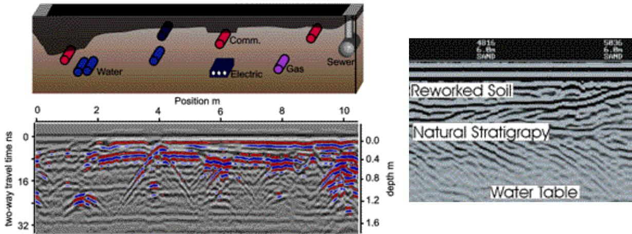
**Figure 5-32. GPR Results: (a) Buried Utility Locations and (b) Soil Profile of Fill over Soil (from EKKO Sensors & Software: [www.senssoft.on.ca](http://www.senssoft.on.ca))**
