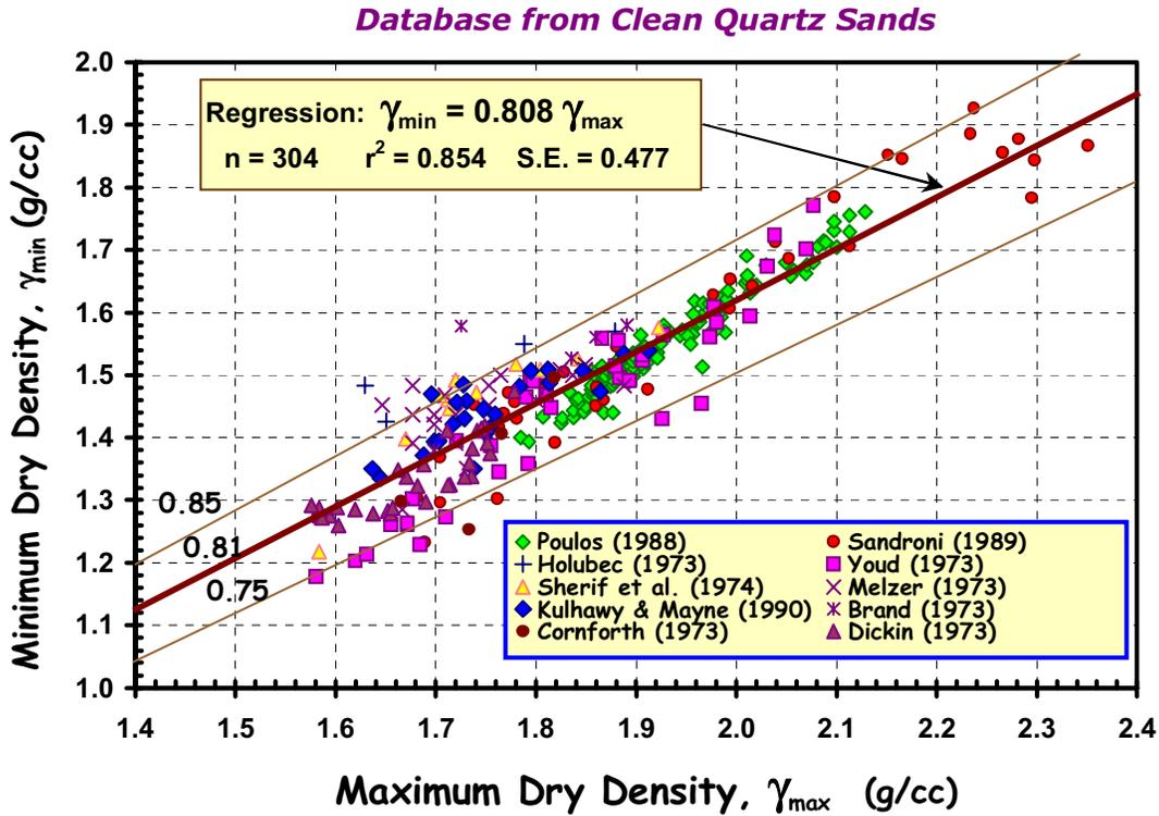
**Figure 9-6. Interrelationship Between Minimum and Maximum Dry Densities of Quartz Sands.**
