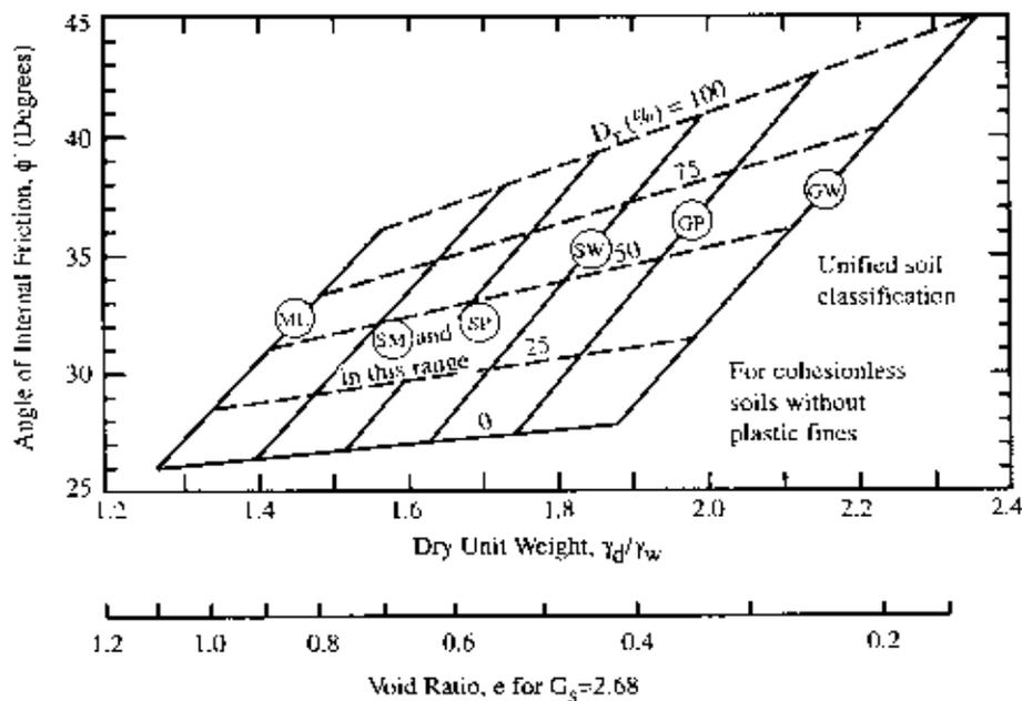
Figure 9-11. Typical Values of  $\phi'$  and Unit Weight for Cohesionless Soils. (NAVFAC DM 7.1, 1982)
