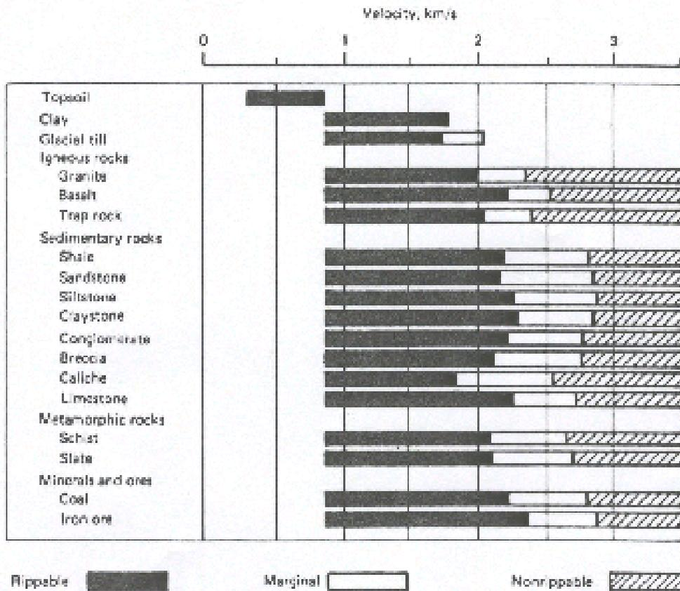
**Figure 10-22. Rippability of Inplace Rock by Caterpillar Dozer Evaluate by P-Wave Velocity. (After Franklin and Dusseault, 1989)**
