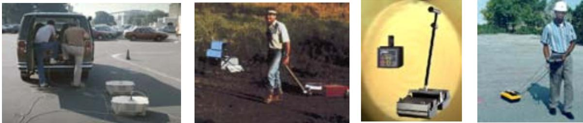
**Figure 5-31. Ground Penetrating Radar (GPR) Equipment from Xadar, GeoVision, and EKKO Sensors & Software.**
