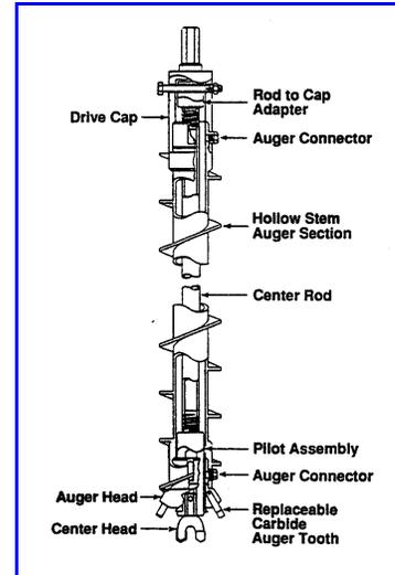
Figure 3-2. Hollow Stem Auger Components (ASTM D 4700).
