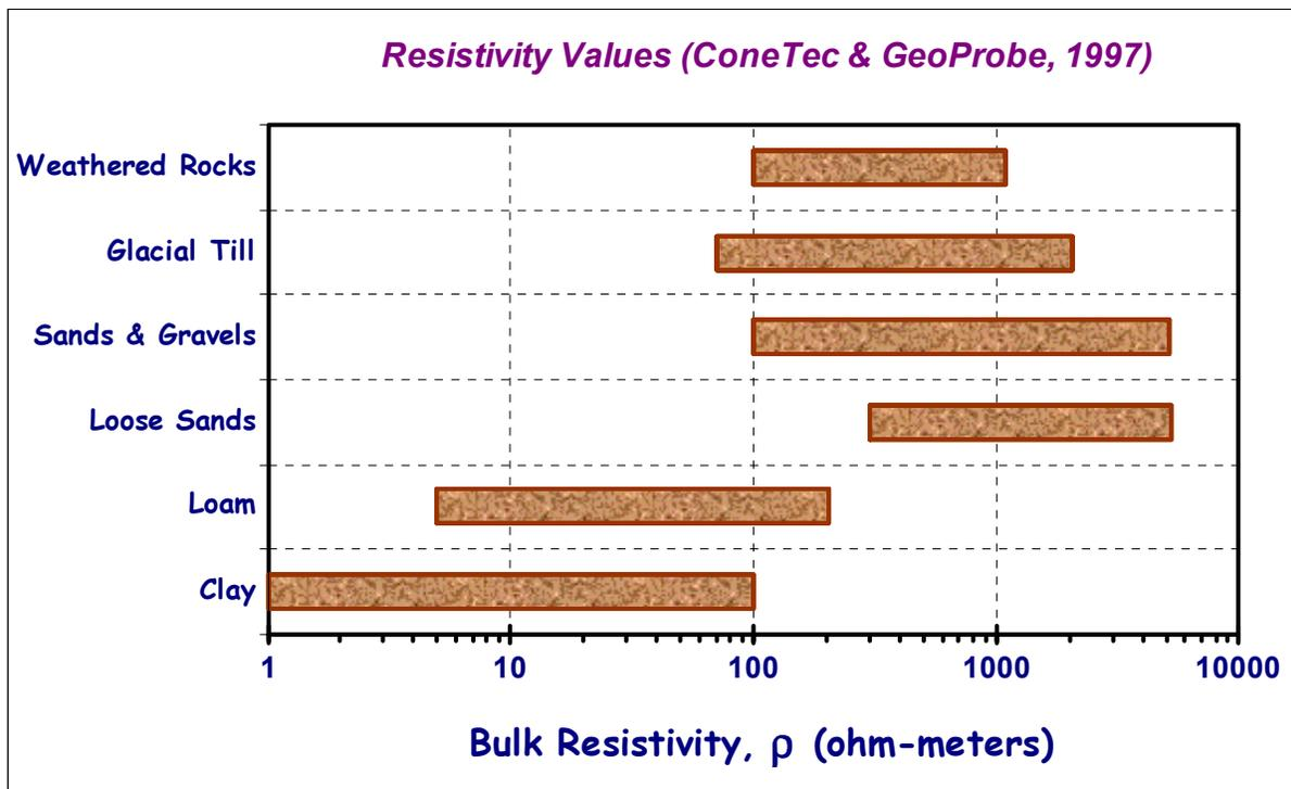
**Figure 5-33. Representative Values of Resistivity for Different Geomaterials.**
