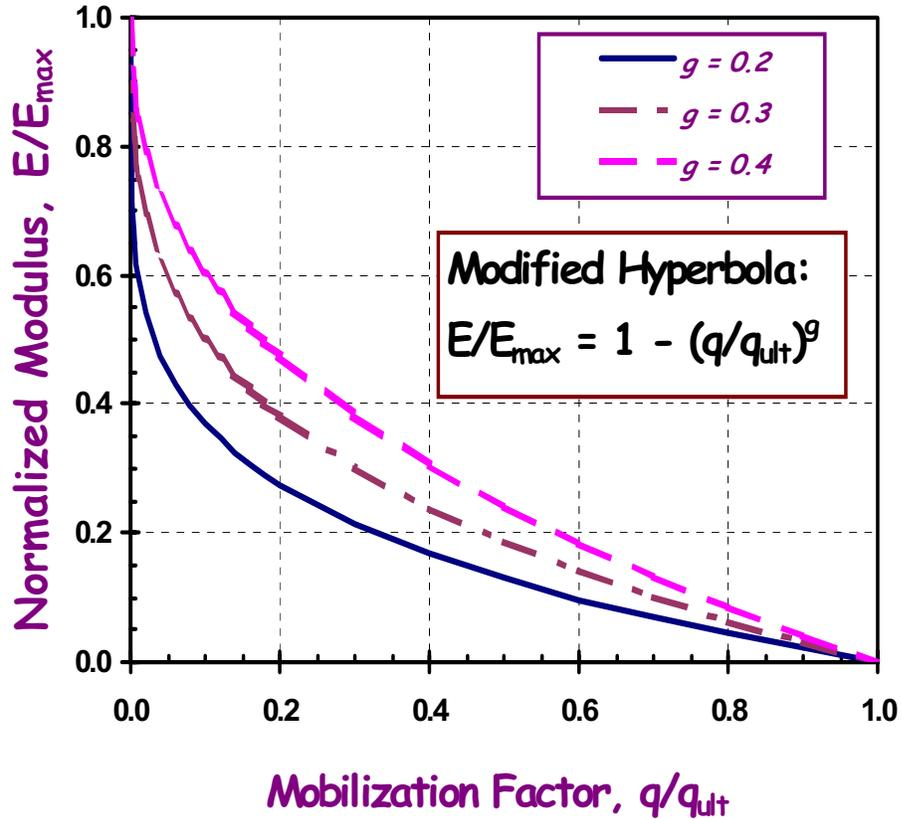
Figure 9-35. Modified Hyperbolas to Illustrate Modulus Degradation Curves (Cases shown for  $f = 1$ ).
