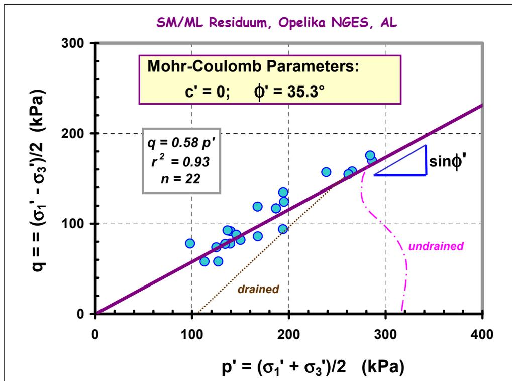
Figure 7-9: Effective q-p' Strength Envelopes for Consolidated Undrained Triaxial Tests.
