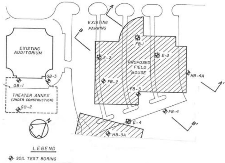
Figure 11-3: Representative Test Location Plan of Completed Soil Boring Locations
