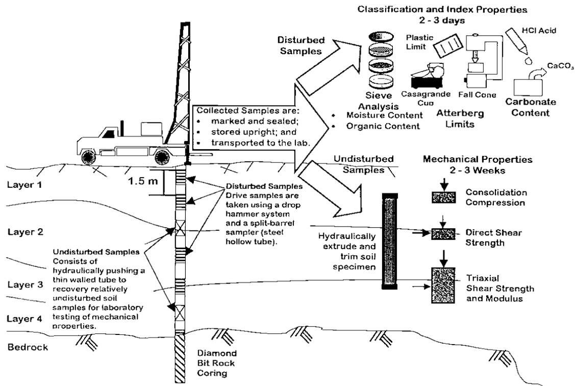
**Figure 9-1. Delineation of Geostatigraphy and Soil & Rock Types by Drill & Sampling Methods.**
