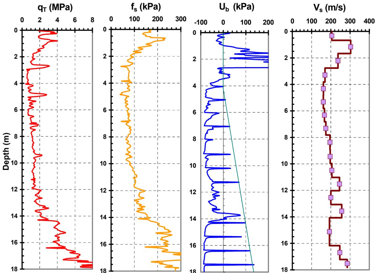
**Figure 5-27. Results of Seismic Piezocone Sounding in Residual Soils in Coweta County, Georgia showing four independent readings with depth. Note: Penetration porewater pressures allowed to dissipate at each rod break.**
