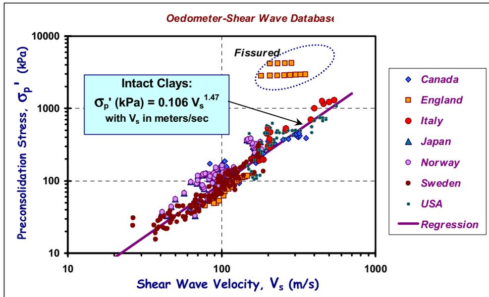
Figure 9-23. Relationship Between Preconsolidation Stress and Shear Wave Velocity in Clays.
