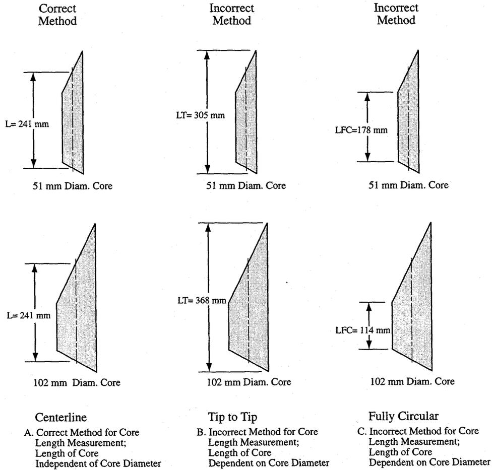
Figure 3-21: Length Measurement of Core RQD Determination
