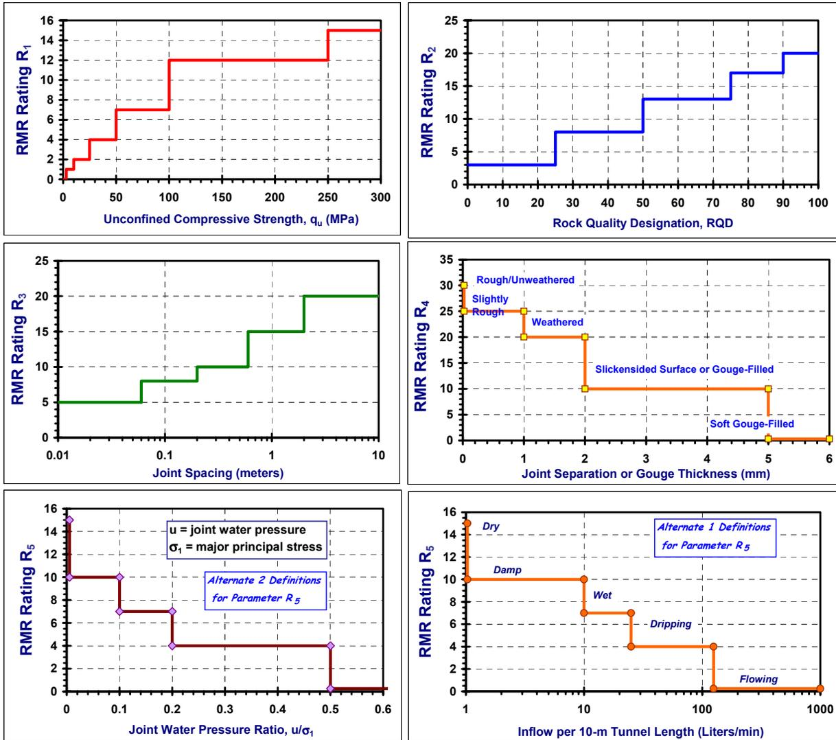
Figure 10-13. The Geomechanics Classification System for Rock Mass Rating (RMR) (after Bieniawski, 1984, 1989).
