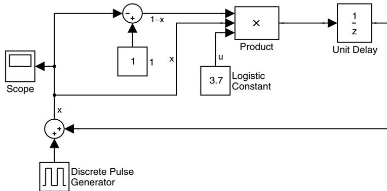
Let's briefly explain how this works. If you ignore the Discrete Pulse Generator block and the Sum block in the lower left for a moment, this model implements the equation
