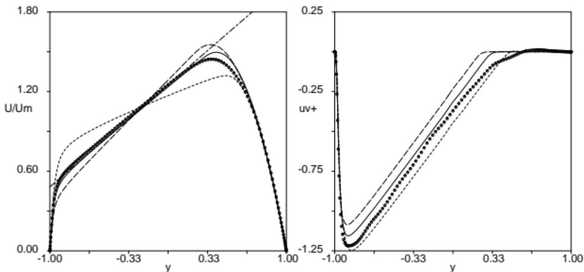
Figure 1: Computed rotating channel flow for  $Ro = 0.77$  compared to DNS of Alvelius & Johansson (2000). Curvature corrected original (---) and recalibrated (—) WJ EARS compared to the non-corrected EARS (— · — ·).  $U' = 2\omega_z^{(r)}$  (---) is also shown. (figure taken from Wallin & Johansson, 2002)
