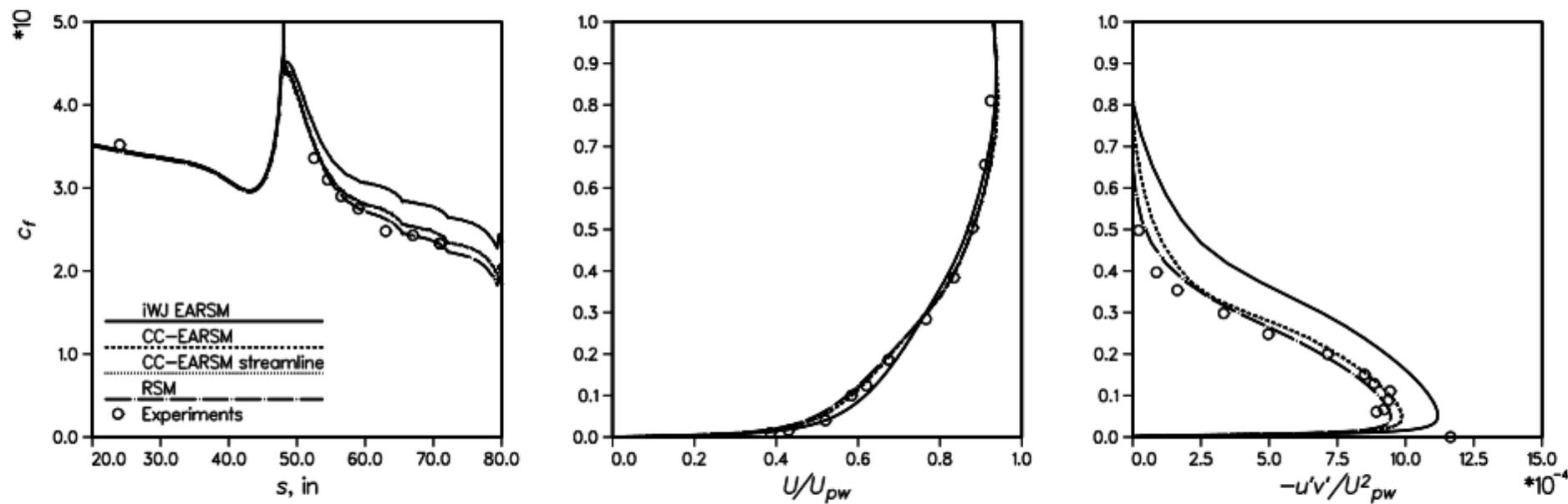
Figure 2: The skin-friction coefficient along the convex wall, the velocity profile and turbulent shear stress at  $s = 71$  in. Experiment by So & Mellor (1973). The stresses are transformed into the local wall-tangential and -normal coordinate system, and  $U_{pw}$  is the theoretical potential velocity on the wall.
