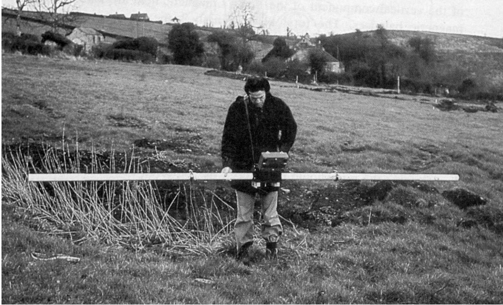
Fig. 4.3 Geonics EM31 ground conductivity meter
